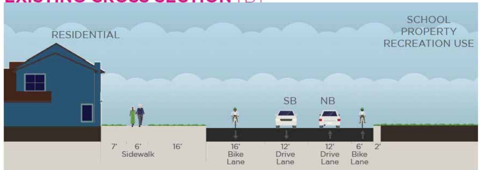
EXISTING CROSS SECTION [B]
