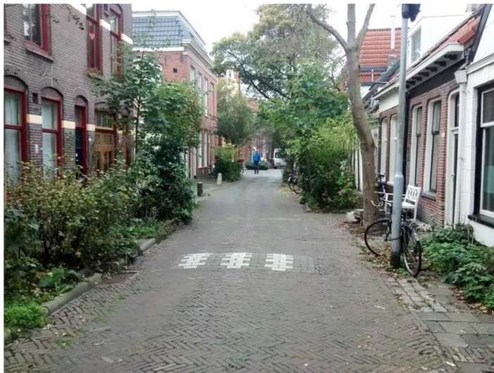
A shared street or "woonerf" in the Netherlands. This street incorporates textured pavement, speed bumps, benches, and greenery. (Source: Alchetron)
