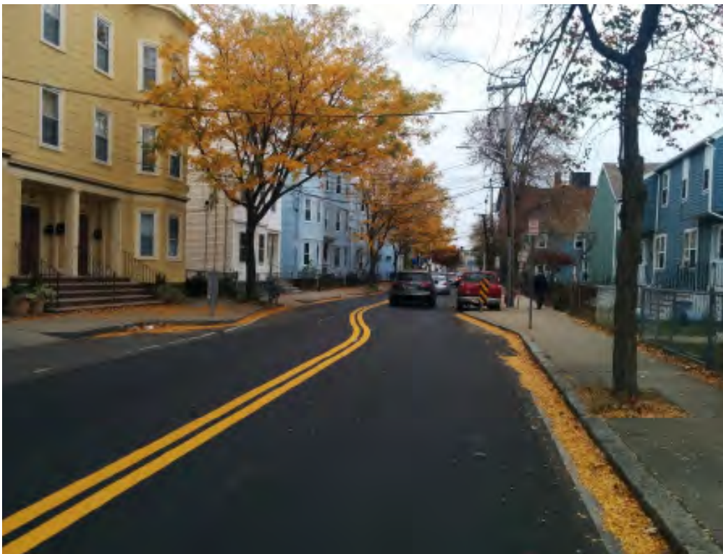
Mid-block deflection through use of on-street parking (Cambridge, MA)
