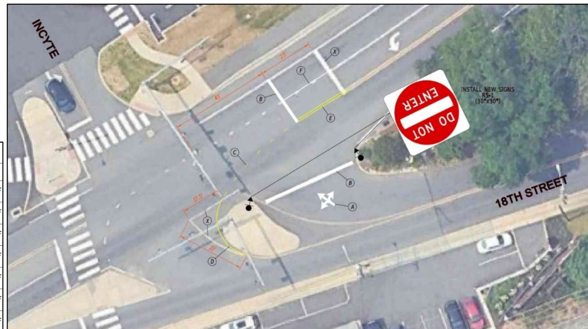
Figure 32. Proposed short-term striping and signage improvements at the ACO and W. 18th Street intersection.
