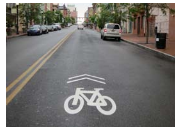
Shared Lane Marking
